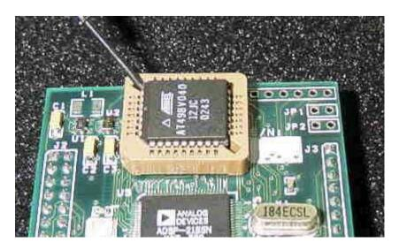
The flash chip should now be completely loose.
