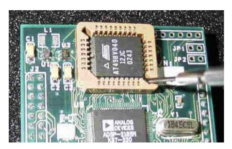
There are two slotted corners in the PLCC socket holding the flash. Carefully insert the screwdriver and pry out a corner of the Flash chip.
